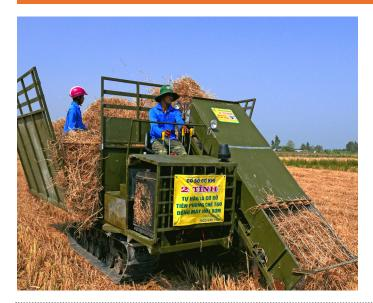
This machine (left photo) is used to collect scattered straw in the field. It is usually self-propelled and is easy to operate.
