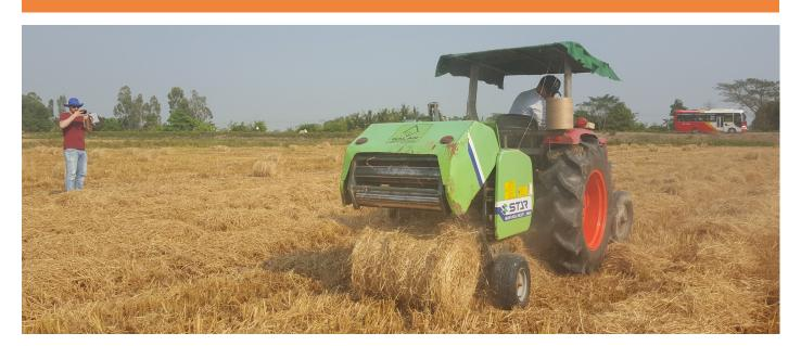
The small-scale roller baler collects and compacts rice straw into round bales. It can be pulled by a tractor or be self-propelled, such as the Japanese STAR baler, pictured above.
