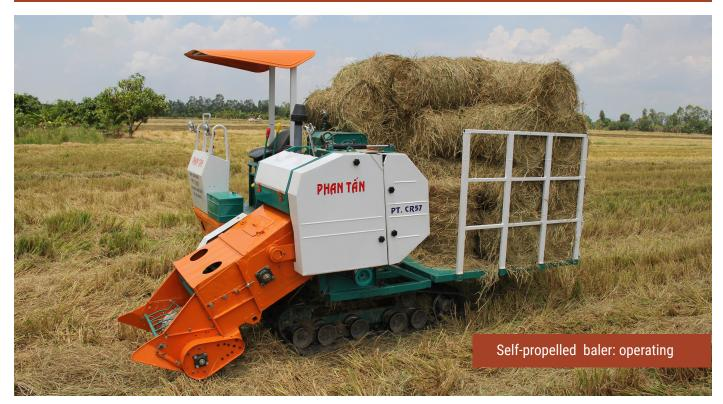
This machine makes bales and transports them to the bund as shown in the photos below. Although it has a higher capacity than the roller baler, its collection capacity is lower because it moves on rubber chain wheels that allows it to be used on wet fields.
