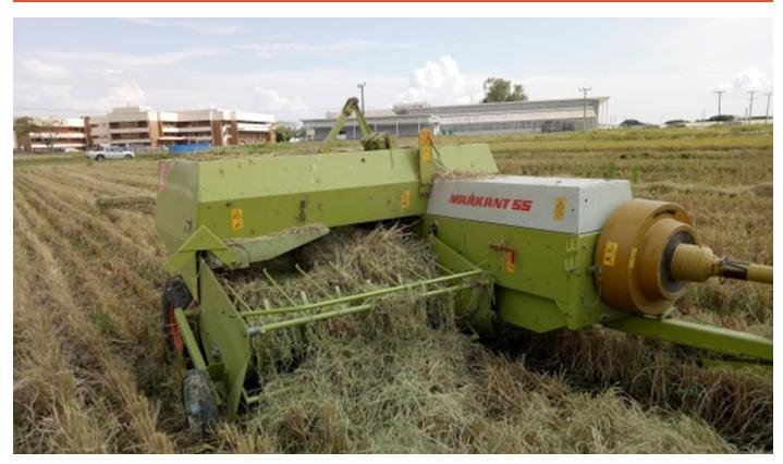
This machine works similar to the roller baler except that it has a piston mechanism that compresses the rice straw into square bales and can operate continuously. This machine is usually pulled by a tractor.
