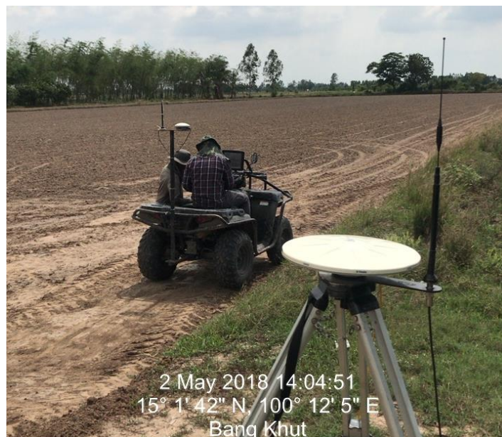
Fig. 17. Conducting field survey with a rover and an RTK base station. (Photo: courtesy of Thanach Songmethakrit)
