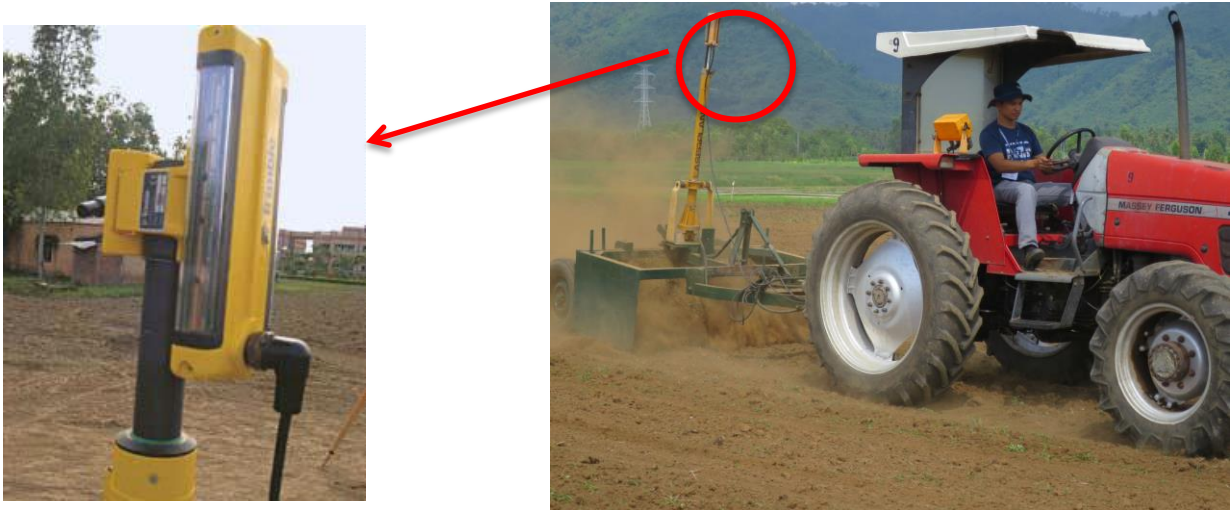
Fig. 7a. Laser receiver mounted on the scraper bucket. Source: Trimble (2015).
