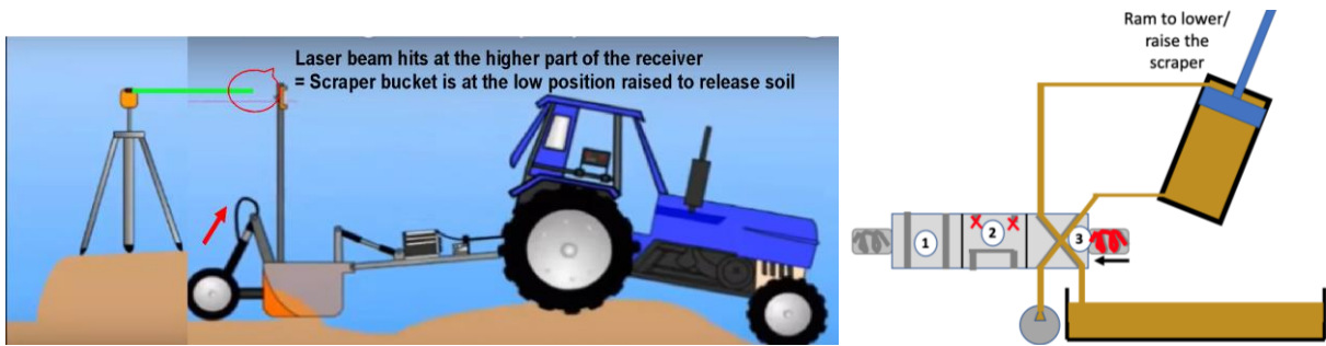
Fig. 11c. Scraper bucket at the “too low” position raised to release soil (left) and the hydraulic valve activated scenario (right)
