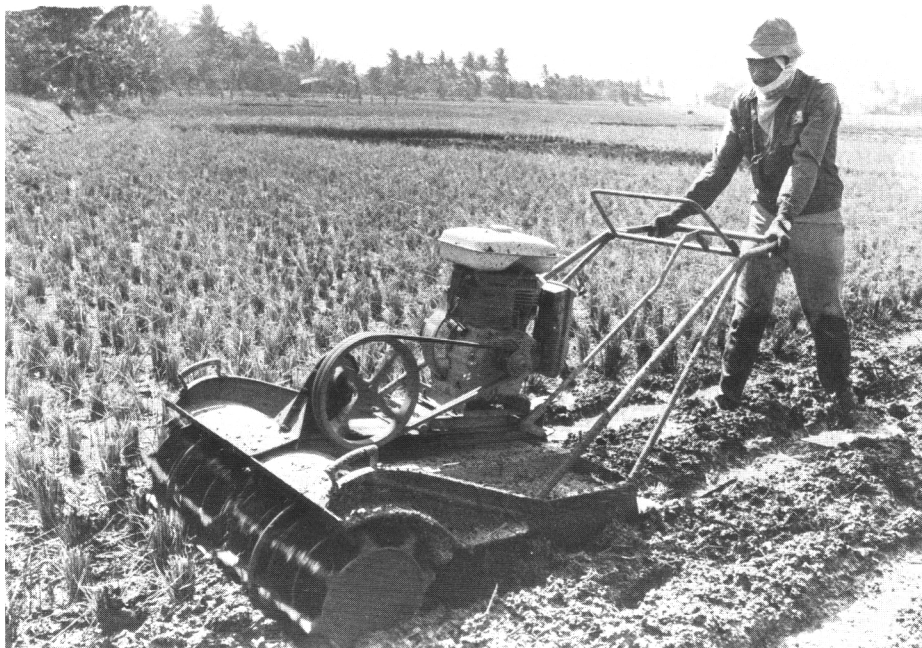
New IRRI hydrotiller (1.m working width) being used to incorporate stubbles in a puddled ricefield.
