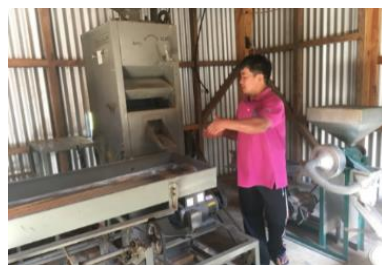
Figure 32. Demonstration of the micro length grader
