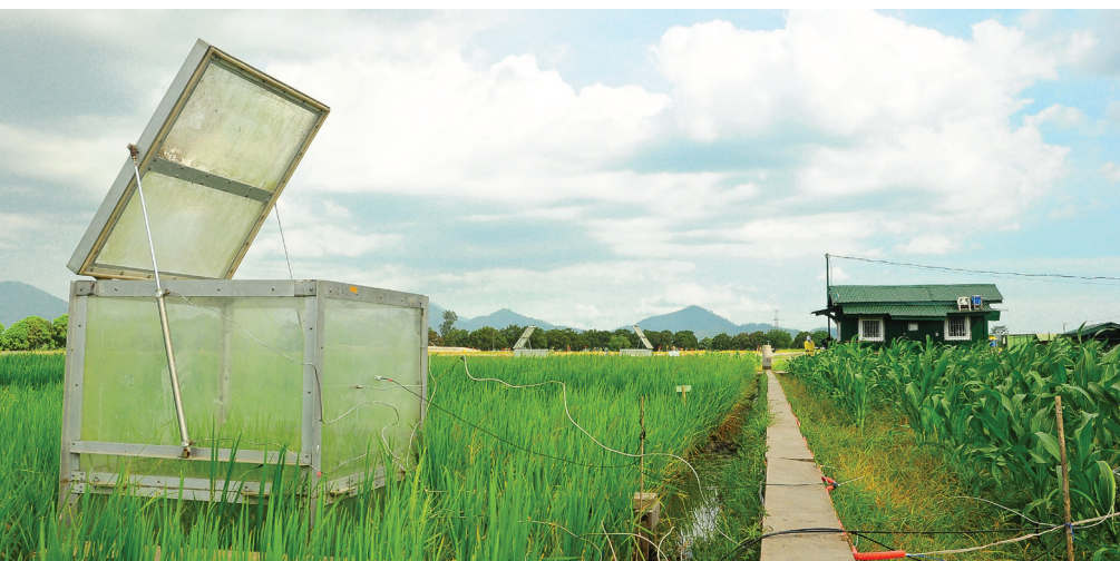
Measuring the invisible. Rice cultivation is one of the primary sources of methane emissions. Scientists use the chambers (above) and the Eddy Covariance (see opposite page) to determine the greenhouse gas emissions of different rice production systems.
