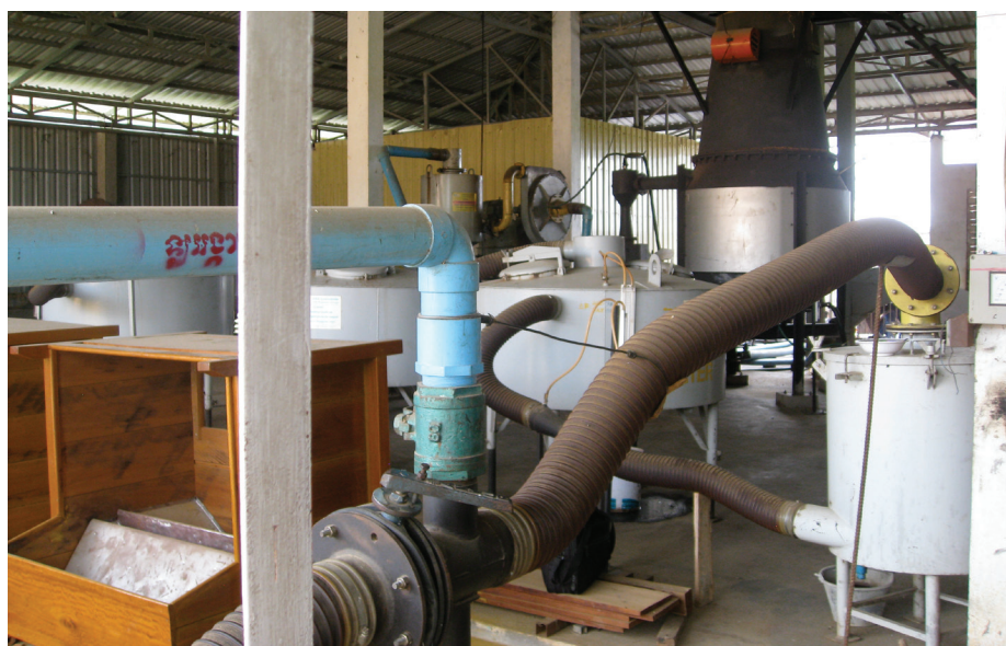
Green power source. A gasifier system not only uses renewable energy from bio-waste products but also doubles as a waste disposal system.
