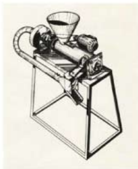
A compact, low-power micro rice mill can process 60-80 kg rice per hour.
