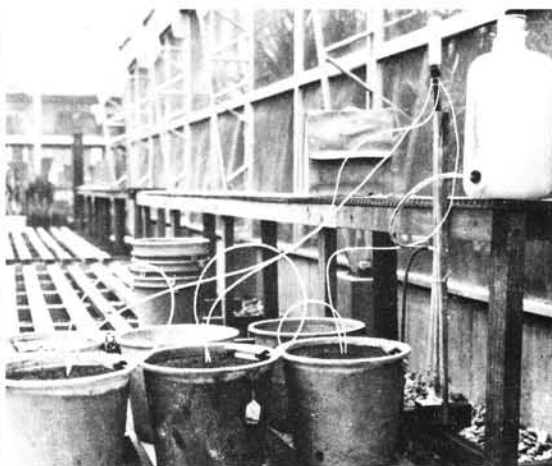
13. Greenhouse set-up for measuring drought tolerance: left photo shows delivery porous cups in each pot and nylon tubing which connects the bubble trap and the sensing tensiometers placed at 10 cm soil depth; right photo shows that each set-up can maintain a predetermined soil moisture tension in three pots.
