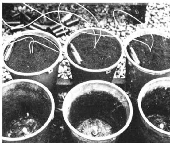
13. Greenhouse set-up for measuring drought tolerance: left photo shows delivery porous cups in each pot and nylon tubing which connects the bubble trap and the sensing tensiometers placed at 10 cm soil depth; right photo shows that each set-up can maintain a predetermined soil moisture tension in three pots.
