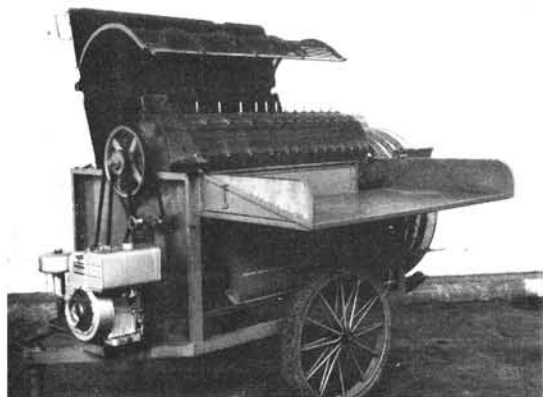
1. Axial flow thresher with cover open and upper concave exposed.
