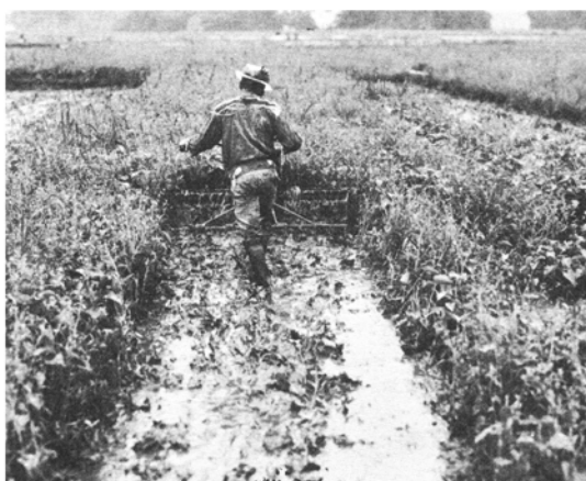
Fig. 2. A hand tiller with cage wheels and comb harrow can prepare soft soils in 3 to 5 passes.
