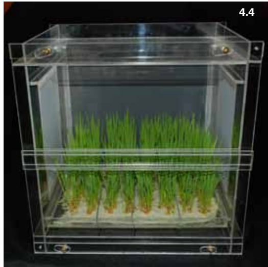
Fig. 4.3. Aluminum rearing/oviposition cage (56.5 cm × 56.5 cm × 91.5 cm) with aluminum wire mesh on three sides, top, and doors for ventilation. Fig. 4.4. Flexi-glass cage (30 cm × 25 cm × 30 cm) with seedling mat.
