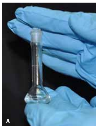
Fig. 9.1. Preparation of stock solution: (A) technical grade insecticide dissolved inside a standard volumetric flask; (B) Erlenmeyer flasks with insecticide dilutions.
