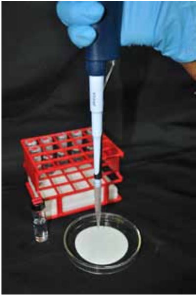
Fig. 11.5. Filter paper treated with the desired ME concentration on a glass petri dish.
