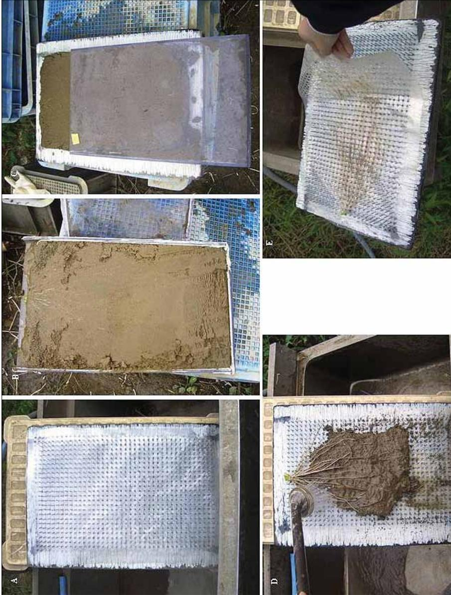
**Fig. 1. A pinboard wrapped in a perforated polyethylene sheet (A). The root box was laid down on a flat surface with removable sidewall removed (B). The box was slid down and the soil was left on the pinboard in between plastic sheets (C). Washing of the root system (D). The root system sandwiched between the sheets (E).**
