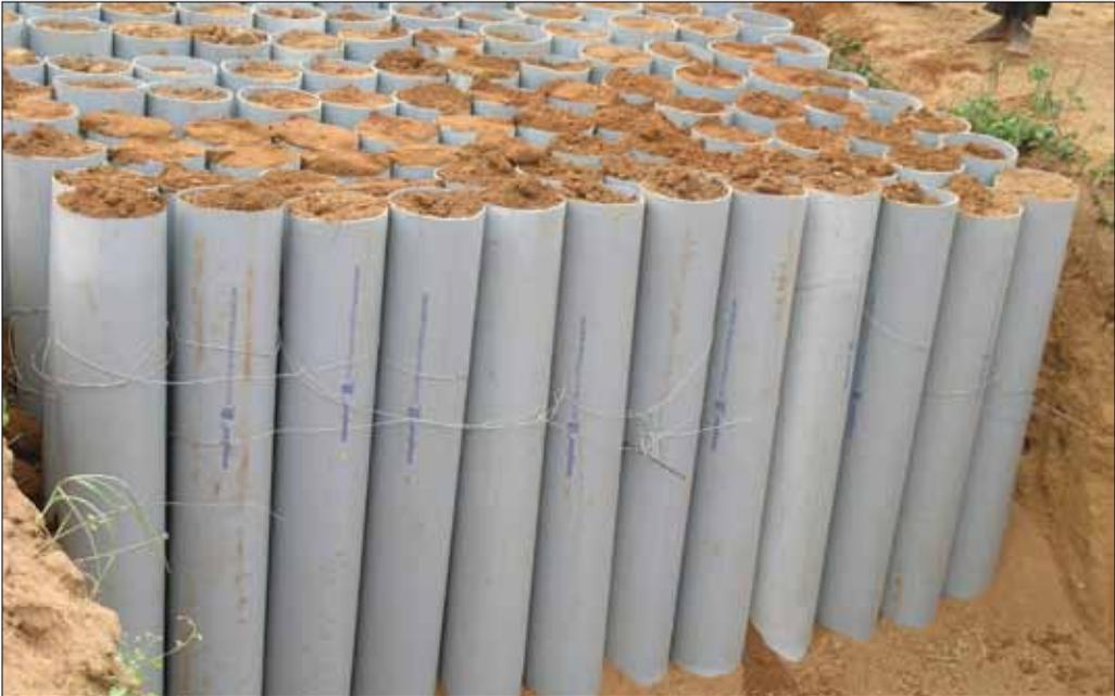
**Fig. 1.** PVC tubes filled with soil, arranged in the pit.
