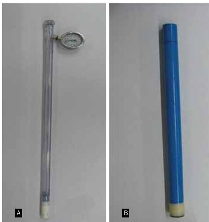
**Fig. 2. Simple tools for characterizing the type of drought stress that occurs in drought field experiments. (A) A tensiometer for measuring soil water potential and (B) a home-made tube well (piezometer or water table tube) that is sealed on the bottom with cotton cloth, and with narrow slits in the side to allow entry of water but prevent filling with mud.**
