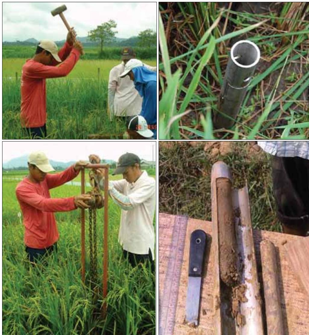
**Fig. 6. (From left to right) Root sampling by soil core: pounding in the core tube, using a wooden block to reduce equipment damage, removal of core tube with a chain block and pulley, and division of soil core to represent 15-cm-depth segments.**
