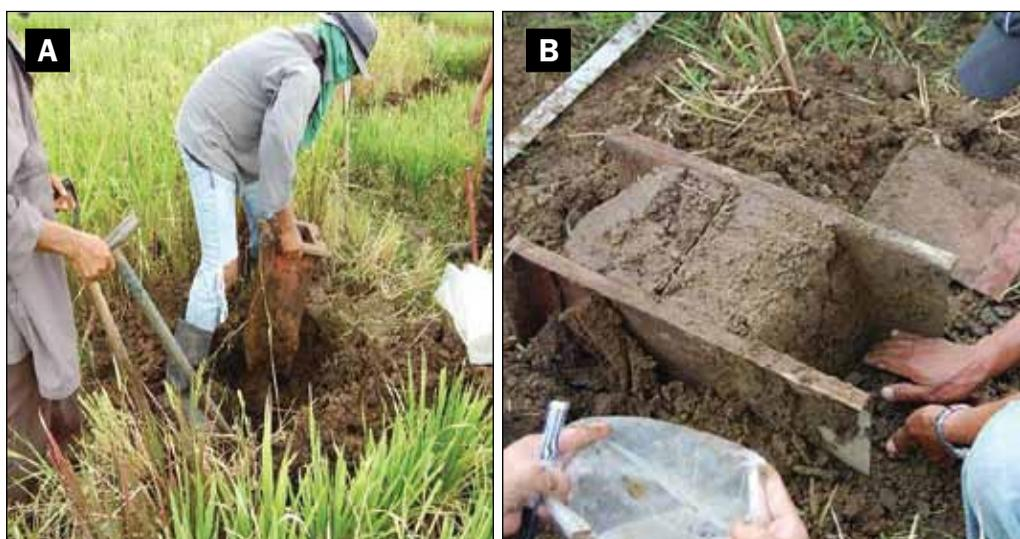
**Fig. 5. (A) A hole is dug in the soil to tilt the monolith sampler before removal from the soil. (B) The side of the sampler is slid off and the soil is divided into 15-cm segments.**
