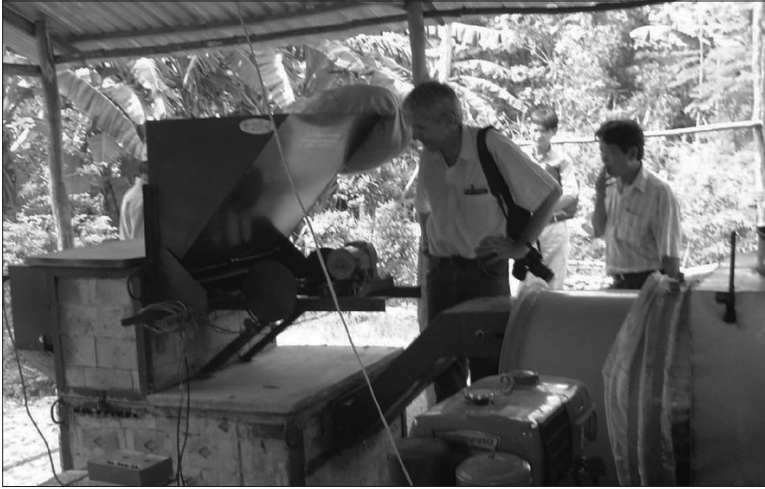
Fig. 8. The automatic rice husk furnace for the SRA-4 reversible flat-bed dryer.
