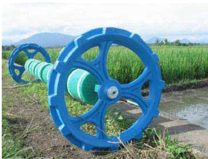
This plastic drum seeder, made in Vietnam, works better with four cylinders than with six.
