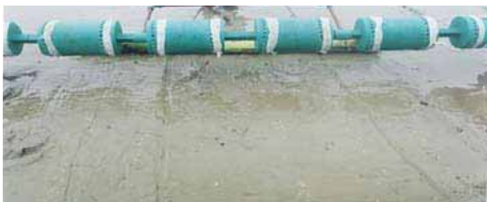
Fig. 3. Sprouted rice seeds planted in lines by using a plastic drum seeder.
