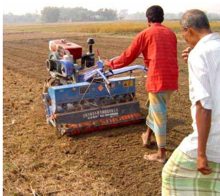
The power tiller and the seed drill in action. Farmers walk behind the drill to monitor the wheat-planting activity.
