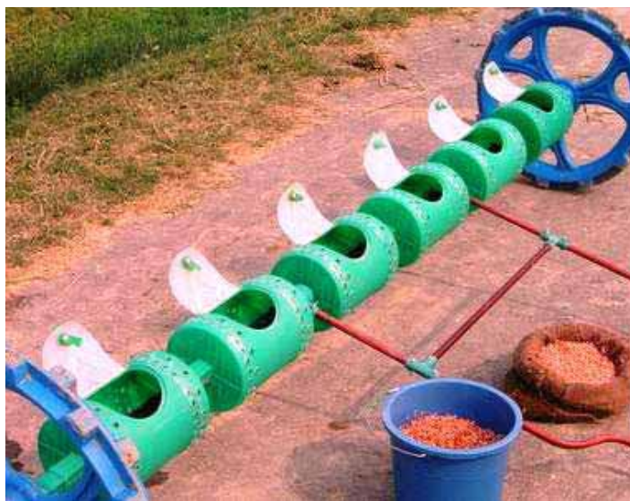
Fig. 1. A Vietnamese-made plastic drum seeder and sprouted rice seeds for planting.
