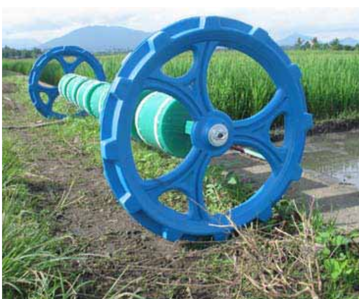
Fig. 1. The plastic drum seeder for direct wet seeding of rice.
