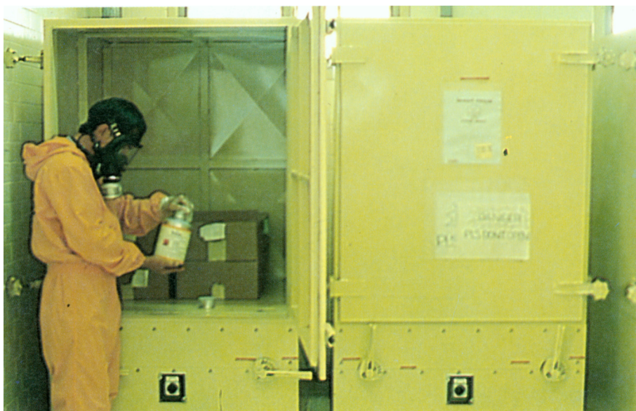
11.3 Fumigation using atmospheric-type fumigation chamber and phosphine.
