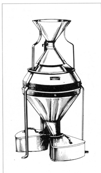
4.3 A conical divider (Boerner type).
