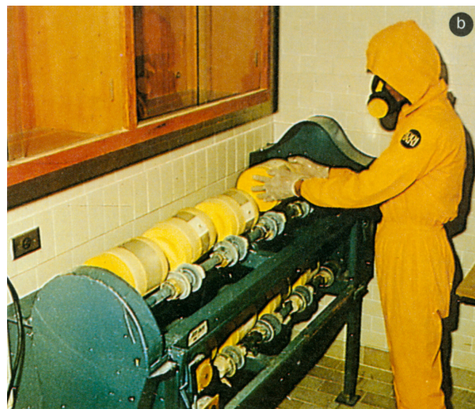
11.2a. Slurry treatment. Small plastic bottle for 50-g seeds and bigger plastic bottle for 100-g seeds. b. Slurry treatment. Big plastic bottle for 1-kilo seeds placed on a roll mill and rotated for 510 min.
