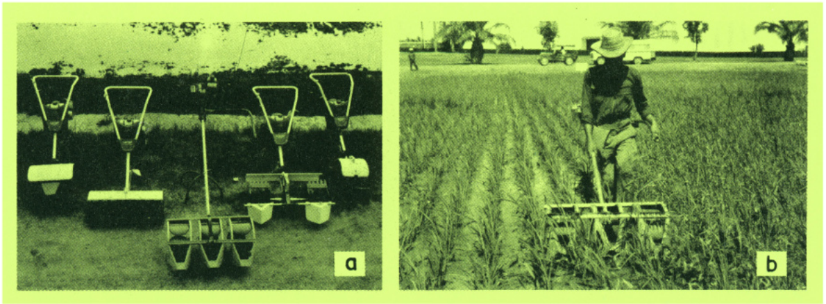
14. a) IRRI 3-row portable power weeder prototype with commercially produced Japanese weeder by Ohtake & Co. b) IRRI 5-row portable power weeder prototype.
