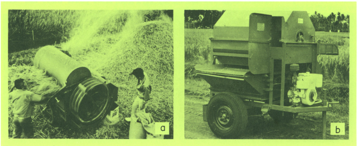
11. IRRI axial-flow thresher: a) original prototype units, and b) latest version.
