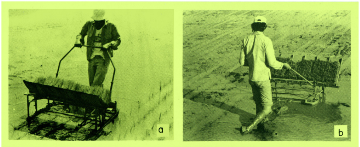
16. a Manually-operated 5-row IRRI transplanter(original design). b) Improved 6-row transplanter.
