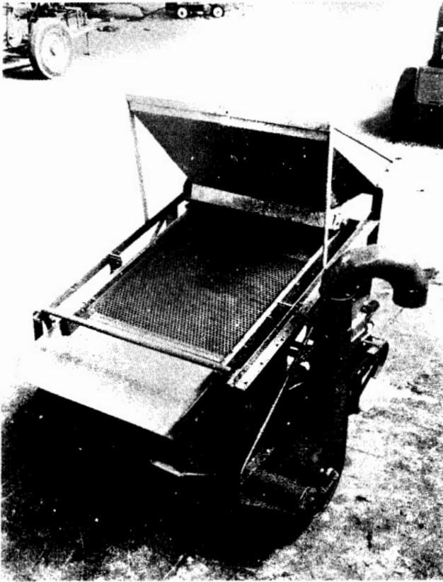
A small paddy cleaner suitable for use jointly by several farmers. (Source: IRRI)
