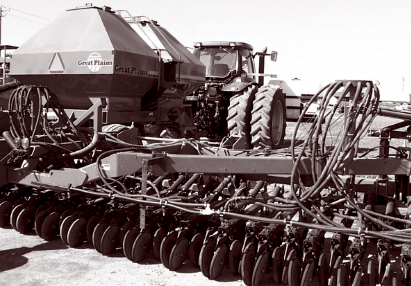
Large-scale mechanized rice farmers in the United States use equipment such as this minimum till air drill that plants 65 rows at a time with a holding capacity of 10,000 pounds of seed. Source: Jay Cockrell, Texas Rice Newsletter .
